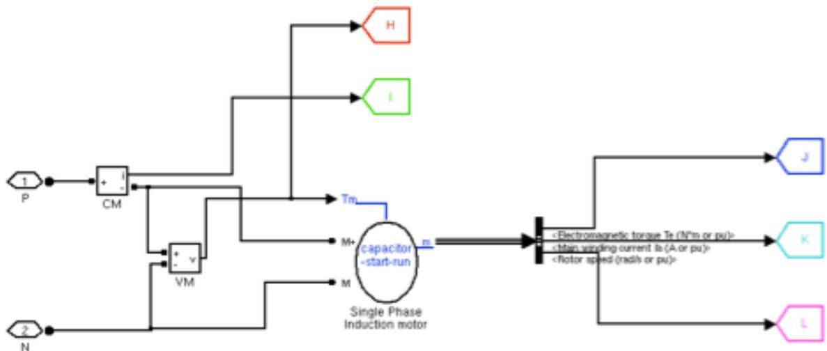
**Fig: 3.6.1** Simulation for single phase induction motor
