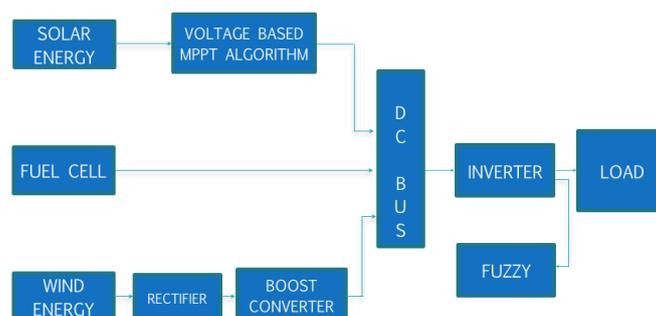
**Fig 4.1** Block diagram of hybrid system
