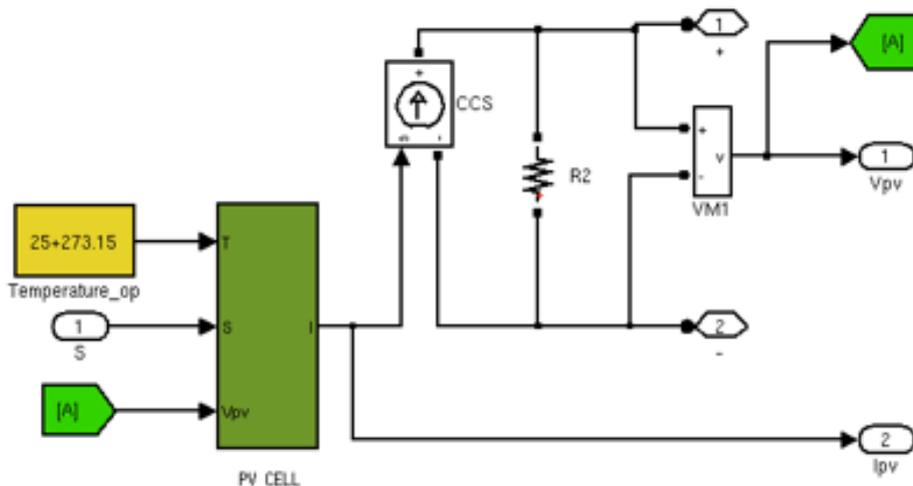
Fig 3.1.2 simulation for photovoltaic
