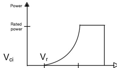
Fig. 3.2.1. Wind turbine characteristics.
