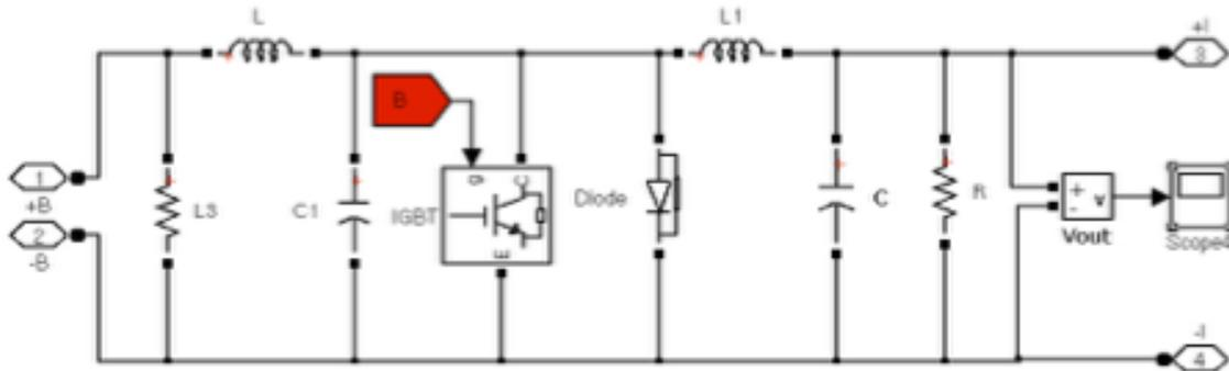
**Fig 3.4.1** Simulation for boost converter
