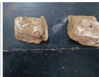
**Figure 17 : Calcium Carbonate precipitation over the bricks**
