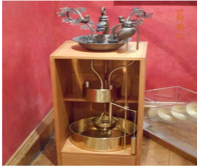
Picture 8. The hydraulic automation of the “chirping birds” and the “returning owl”.
