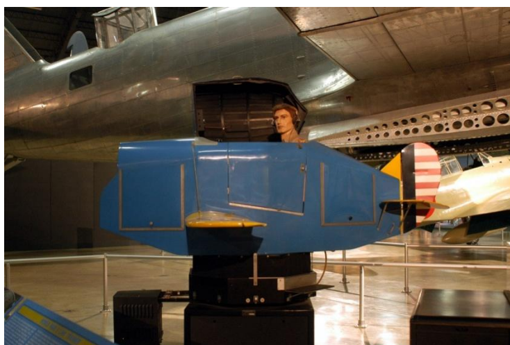
Figure2 : Link Trainer in the World War II Gallery at the National Museum of the USAF
