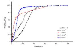
Fig.6.The degradation degree of different initial concentrations of AR44 in presence of  $5.0 \times 10^{-2}$  M  $H_2O_2$ ,  $[Fe^{2+}] = 1.0 \times 10^{-3}$  M in Fenton process at pH 3.0.
