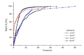
Fig.14.The degradation degree of different initial concentrations of AR44 in presence of  $5.0 \times 10^{-2}$  M H<sub>2</sub>O<sub>2</sub> and [Fe<sup>2+</sup>] =1.0x10<sup>-3</sup> M in photo-Fenton process and pH 3.0.
