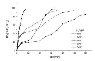
Fig.9.The degradation degree of  $[AR44] = 1.0 \times 10^{-5}$  M with different initial concentrations of  $H_2O_2$  in presence of  $[Fe^{3+}] = 1.0 \times 10^{-3}$  M, in Fenton-like process and pH 3.0.
