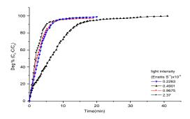
Fig.21.The degradation degree of AR44 at different light intensity in presence of  $7.0 \times 10^{-5}$  M AR44,  $5.0 \times 10^{-2}$  M H<sub>2</sub>O<sub>2</sub>,  $5.0 \times 10^{-3}$  M Fe<sup>3+</sup>, in photo-Fenton like process and pH 3.0.
