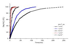
Fig.11.The degradation degree of different initial concentrations of  $Fe^{2+}$  in presence of 5.0 x10<sup>-2</sup> M H<sub>2</sub>O<sub>2</sub> and [AR44] =7.0x10<sup>-5</sup>M, in photo-Fenton process and pH 3.0.
