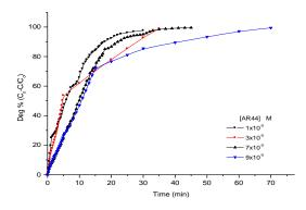
Fig.15.The degradation degree of different initial concentrations of AR44 in presence of  $5.0 \times 10^{-2} \text{ M}$  H<sub>2</sub>O<sub>2</sub> and [Fe<sup>3+</sup>] =1.0×10<sup>-3</sup> M, in photo-Fenton- like process and pH 3.0.
