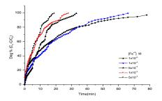
Fig.10.The degradation degree of different initial concentrations of  $Fe^{2+}$  in presence of 5.0 x10<sup>-2</sup> M H<sub>2</sub>O<sub>2</sub>, [AR44] =1.0x10<sup>-5</sup> M in photo-Fenton process and pH 3.0.
