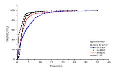
Fig.19.The degradation degree of AR44 at different light intensity in presence of  $7.0 \times 10^{-5}$  M AR44,  $5.0 \times 10^{-2}$  M H<sub>2</sub>O<sub>2</sub>, $5.0 \times 10^{-3}$  M Fe<sup>2+</sup> in photo -Fenton process and pH 3.0.
