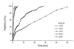
Fig.16.The degradation degree of different initial concentrations of  $H_2O_2$  in presence of [AR44] =1.0x10<sup>-5</sup>M, [Fe<sup>2+</sup>] =1.0x10<sup>-3</sup>M, in photo-Fenton process and pH 3.0.
