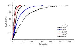
Fig.13.The degradation degree of different initial concentrations of  $\text{Fe}^{3+}$  in presence of  $5.0 \times 10^{-2} \text{ M}$  H<sub>2</sub>O<sub>2</sub> and [AR44] =7.0×10<sup>-5</sup> M, in photo-Fenton like process and pH 3.0.
