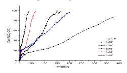
Fig.4.The degradation degree of different initial concentrations of Fe<sup>3+</sup>in presence of 5.0  $\times 10^{-2}$  M H<sub>2</sub>O<sub>2</sub>, [AR44] =1.0 $\times 10^{-5}$  M in Fenton-like process at pH 3.0.
