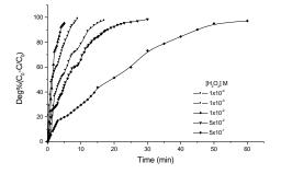
Fig.17.The degradation degree of different initial concentrations of  $H_2O_2$  in presence of [AR44] =1.0x10<sup>-5</sup>M, [Fe<sup>3+</sup>] =1.0x10<sup>-3</sup>M, in photo-Fenton like process and pH 3.0.
