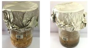
Figure 24: Dried Substrates soaked overnight – SB; OC
