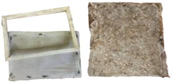
13A 13B Figure 13A: Mould and Deckle used for Paper Laying Figure 13B: Sample Laid on Mould and Deckle
